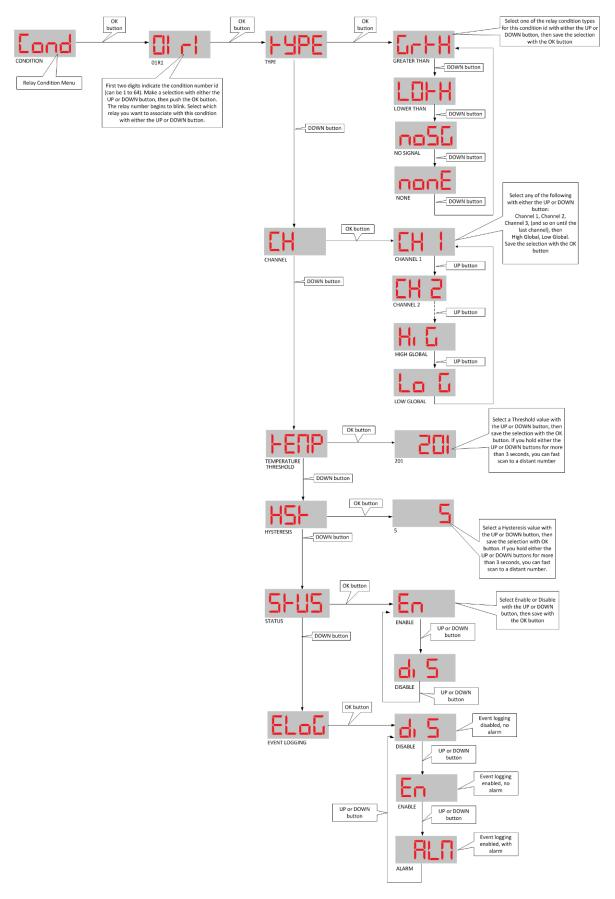
The Relay Condition menu is the most complex of the menus, with a logic path five-level deep. This allows you to set conditions that will trigger a relay, and by extension an automated process, when the desired conditions are met.
