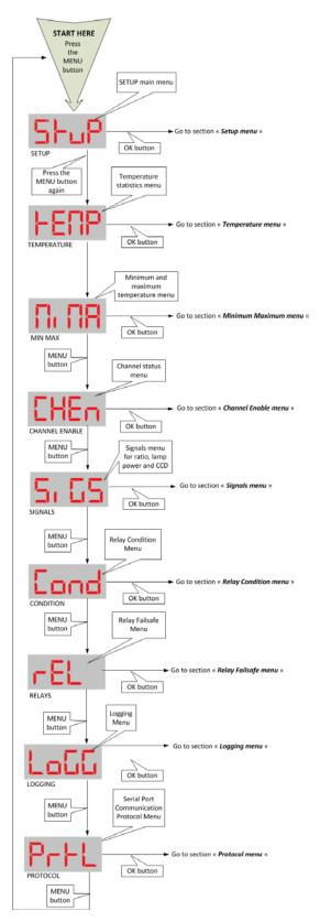
This page provides a diagram of the sub-menus for the 408XT model (with Ethernet):
