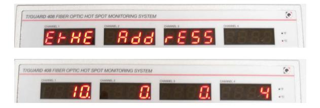
• Click either the third or fourth UP/DOWN button once, and the "IP" submenu will be displayed blinking along with the current "STATIC" configuration;
