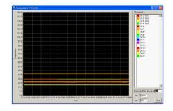
Adjust the "Refresh Rate" and Min / Max to suit your viewing needs. The minimum refresh rate is 0.2 second in OptiLink; however the *T/Guard 408* will send temperature data once every two seconds.
