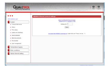
The device address id can be modified here. This id must be between 1 and 247 (0 is not valid, and values from 248 to 255 are tolerated although as per the Modbus protocol they are illegal). It is suggested to always use id=1, even when multiple *408XT* units are networked together, as then the device IP address is in practice the real id differentiator.
