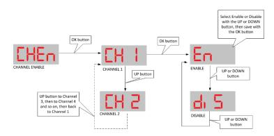
In this menu, you can enable or disable a channel from displaying a temperature. You might want to do this if a fiber optic probe was not hooked up (values for this channel do not apply) or if a probe was broken along the way and thus the displayed temperature is known to be incorrect.
