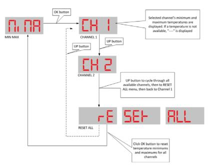
Here, you can view at a glance what the minimum and maximum temperatures measured were for each available channel.
