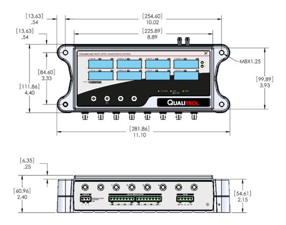
Mechanical details for the 10 to 16 channel version (only height view is shown, as other dimensions are the same as for the 8-channel version, shown above):
